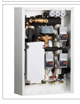
Two pre-packaged systems called: "2 mixed zones kit" and "2 mixed zones and 1 direct zone kit". They are comprised of 2 separate hydraulic manifolds (flow/return) + by-pass, thermometers to read the temperatures, motorised mixing valves, low energy consumption electro pumps and expansion boards for electric management.
