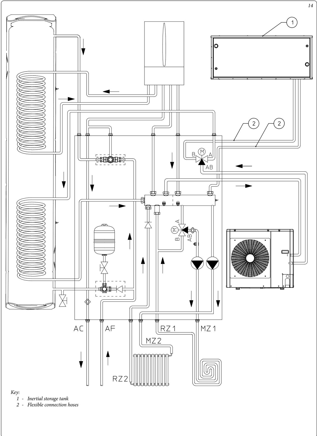
**3.6 RECESSED INERTIAL STORAGE TANK HYDRAULIC DIAGRAM - TRIO CONNECTION WITH MAGIS PRO.**
