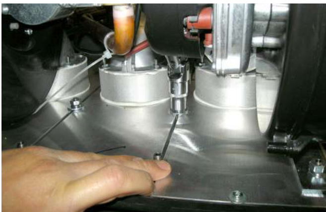
- Take out screws "A" from each element (with 13 mm socket key).
