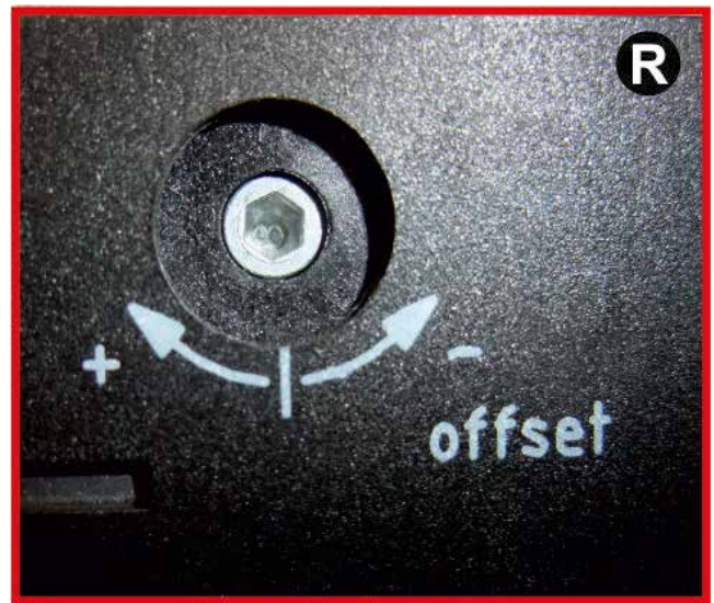
(R) MINIMUM POWER ADJUSTMENT SCREW
