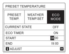
When the cursor is on "START" or "END", you can use "◀", "▶", "▼", "▲" to scroll and "▼" and "▲" to adjust the time.
