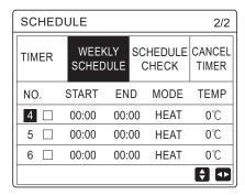
Use "◀", "▶", "▼", "▼" to scroll and adjust the time, the mode and the temperature. Several timer settings can be made, including start and end time, mode and temperature. The Heat mode, Cool mode and DHW mode are included.
