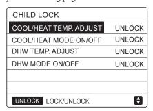
Use "▼" and "▲" to scroll and "ON/OFF" to select LOCK or UNLOCK.
