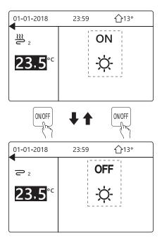
Use the control panel to switch the DHW unit on or off. Press "▶" and "▼" on the home page, the black cursor will appear:
