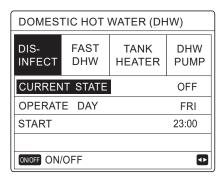
Use "◀", "▶", "▼", "▲" to scroll and "▼" and "▲" to adjust the parameters to set "OPERATE DAY" and "START". If OPERATE DAY is set at FRI. and START is set at 23:00, the disinfect function will activate on Friday at 23:00.
