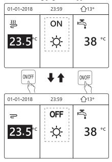
Use the room thermostat to switch space heating or cooling on or off.
