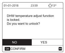
The DHW mode cannot be activated or deactivated when the DHW MODE ON/OFF function is locked. If you try to activate or deactivate the DHW mode when the DHW MODE ON/OFF function is locked, the following page will appear:
