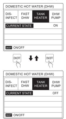
Use the "ON/OFF" key to select activated (ON) or deactivated (OFF). Use "BACK" to exit.
