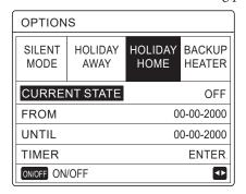
Use the "ON/OFF" key to select activated (ON) or deactivated (OFF) and use "◀", "▶", "▼", "▲" to scroll and adjust. If CURRENT STATE is OFF, HOLIDAY HOME is OFF.
