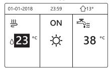
• If the cursor is on the temperature, use " $\blacktriangleleft$ " and " $\blacktriangleright$ " to select and use " $\blacktriangledown$ " and " $\blacktriangle$ " to adjust the temperature.
