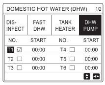
Use "◀", "▶", "▼", "▲" to scroll and use "▼" and "▲" to adjust the parameters.
