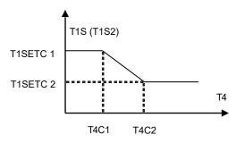
State: in the setting of the control panel, if T4C2 < T4C1, exchange their value; if T1SETC1 < T1SETC2, exchange their value
