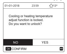
The COOL/HEAT MODE ON/OFF cannot be activated or deactivated when the function is locked. If you try to activate or deactivate COOL/HEAT MODE ON/OFF when the function is locked, the following page will appear:
