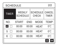
• Use "◀", "▶", "▼", "▲" to scroll and use "▼" and "▲" to adjust the time, the mode and the temperature.
