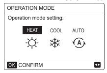
• You may select three modes, namely HEAT, COOL and AUTO. Use "◀" and "▶" to scroll, press OK to select. If you do not press OK and you exit the page by pressing BACK, the mode will remain operational if the cursor was moved to the operation mode.
